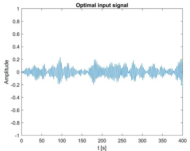
Fig. 3. Optimal input design using D-optimality criteria
