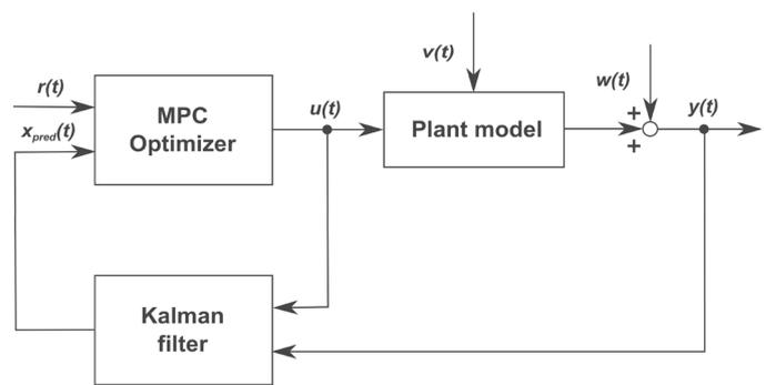
Fig. 7. Block diagram of the system and controller
