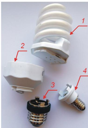
Fig. 10. CFL with interchangeable elements: 1 – discharge pipes, 2 – stabilization-ignition electronic system, 3 and 4 – E27 and E14 cap.
