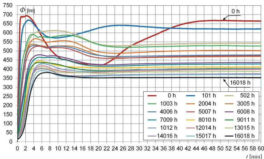
(a) in absolute values during one-hour measurement in the integrating sphere
