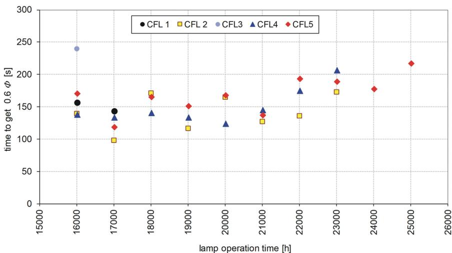
Fig. 8. Time after which individual lamps reach 60% of the luminous flux after time of operation longer than 16 000 h (marks CFL 1 to CFL 5 are used only for distinction of a given Compact Fluorescence Lamp).
