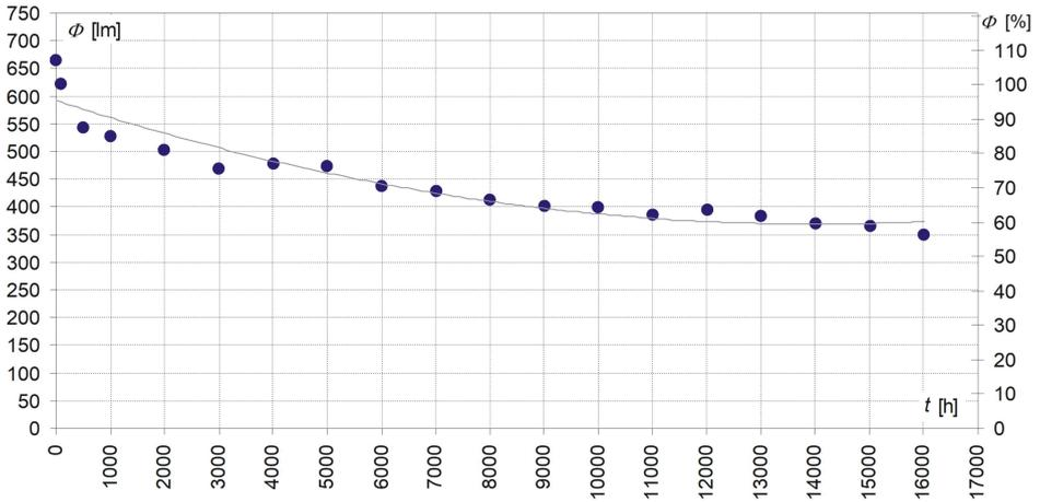
Fig. 5. The average values of the luminous flux as a function of operation time –  $\Phi = f(t)$ .
