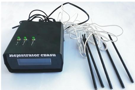
(a) The real view of the recorder registering the exact time of end of lamp lifetime.
