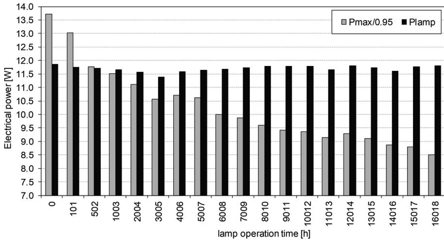
Fig. 9. Illustration of influence of operation time of CFLs on: a) maximum power of lamp to be marked as “energy saver” ( $P_{max}/0.95$ ), b) power of lamp ( $P_{lamp}$ ).
