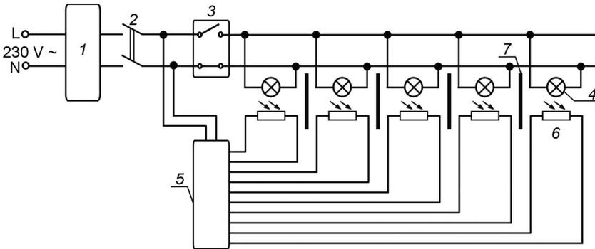
Fig. 3. Scheme of supply circuit for conducting the aging process: 1 – voltage stabilizer, 2 – power switch, 3 – time switch, 4 – tested light sources, 5 – time recorder, 6 – photoresistor, 7 – shutter.
