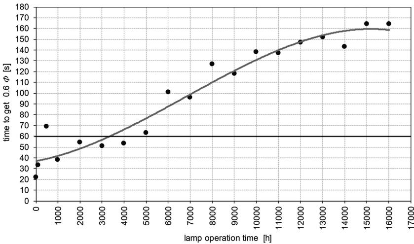
Fig. 7. Time after which the CFLs reach 60% of total luminous flux.
