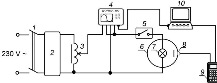
Fig. 1. System for lighting parameters measurement: 1 – power switch, 2 – voltage stabilizer, 3 – autotransformer, 4 – power analyser, 5 – time switch, 6 – integrating sphere (Ulbricht sphere), 7 – light source tested, 8 – photometric head, 9 – luxmeter, 10 – computer PC.
