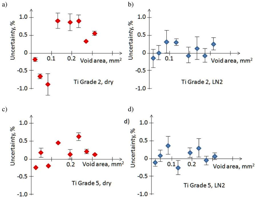
Fig. 7. Uncertainty of measured void area vs. nominal void area (for successive infeeds).
