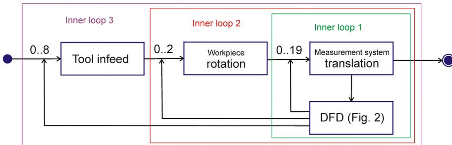
Fig. 1. Measurement state transition diagram of producing a single thread.
