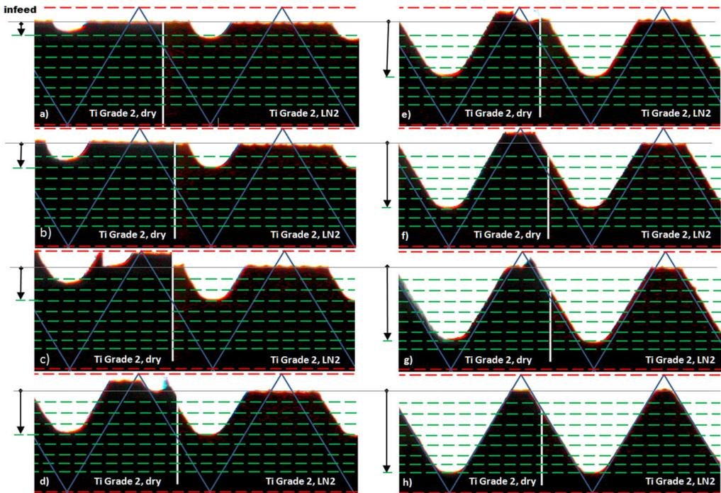
Fig. 4. Optical images of the thread contour for Ti Grade 2 in dry and cryogenic tests.
