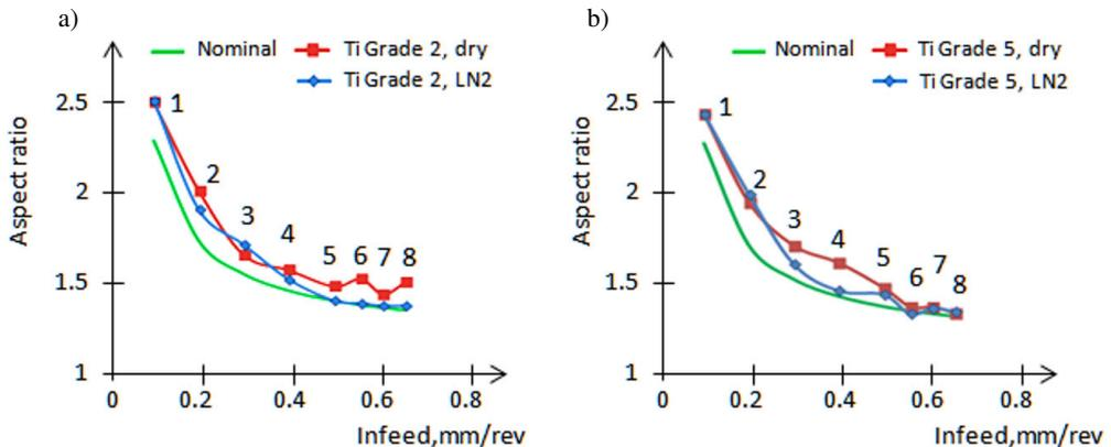
Fig. 8. Measured aspect ratio vs. infeed in thread turning tests of Ti Grade 2 and Ti Grade 5 alloys.
