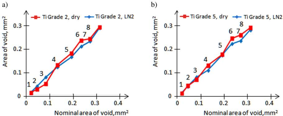
Fig. 6. Measured area of void vs. nominal area of void in thread turning tests of Ti Grade 2 (a) and Ti-6Al-4V alloy (b).
