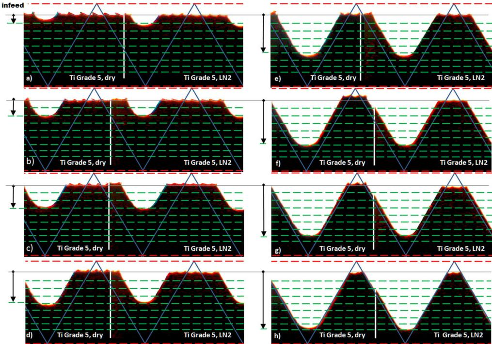
Fig. 5. Optical images of the thread contour for Ti-6Al-4V alloy in dry and cryogenic tests.
