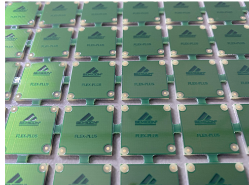
Fig. 3. View of the tested PCB made of a FR4 laminate.
