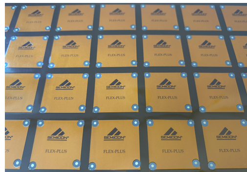
Fig. 4. View of the tested PCB made of a polyimide AP8525 laminate.
