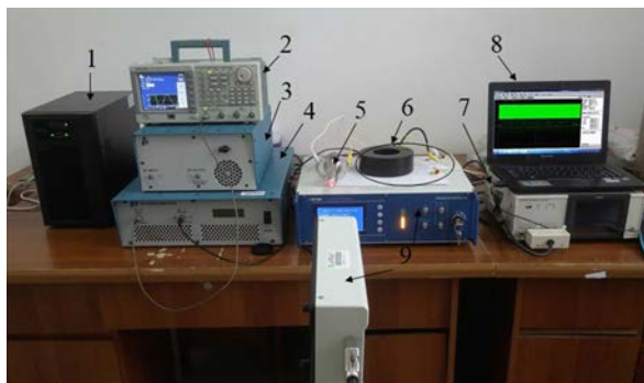
Fig. 14. Testing platform: 1 – uninterruptible power supply, 2 – signal generator, 3 – impedance matching, 4 – power amplifier, 5 – the prototype, 6 – transformer with compensation components, 7 – impedance analyzer, 8 – PC, 9 – laser Doppler vibrometer.
