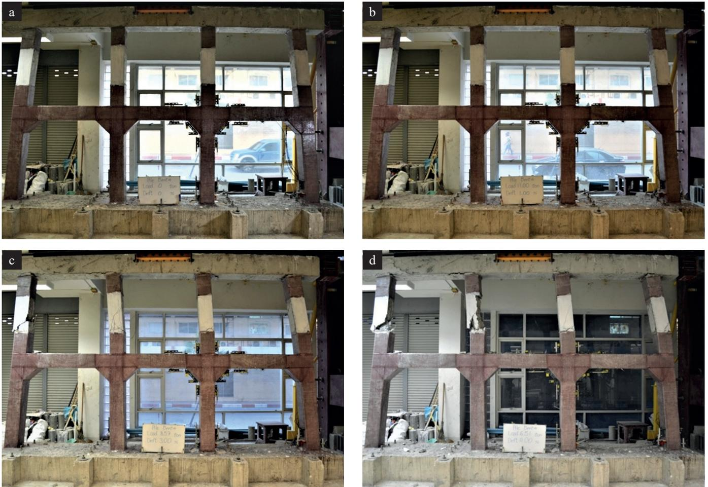
Fig. 14. Damage to the bridge pier P-03 at drift level of: a) 0.50%, b) 1.25%, c) 2.00%, d) 4.00%
