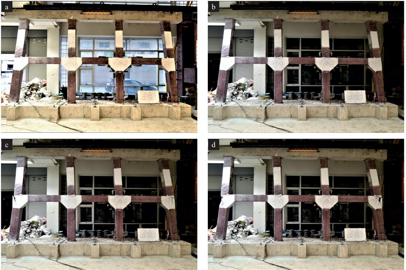
Fig. 12. Damage to the bridge pier P-02 at the lateral drift of: a) 0.50%, b) 0.75%, c) 1.00%, d) 1.50%
