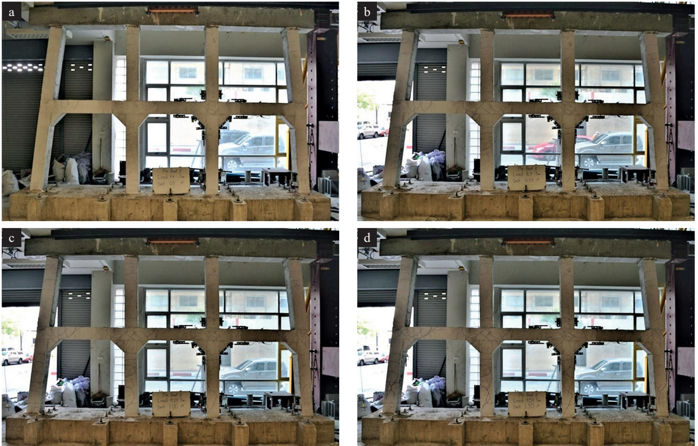
Fig. 10. Damage to the bridge pier P-01 at the lateral drift of: a) 0.50%, b) 0.75%, c) 1.00%, d) 1.50%
