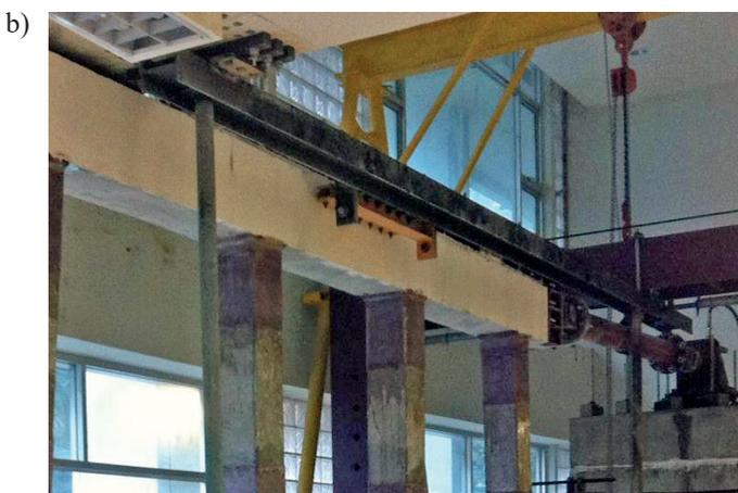
Fig. 8. a) Loading setup (units in mm), b) Lateral supports to prevent out-of-plane movement of bridge piers
