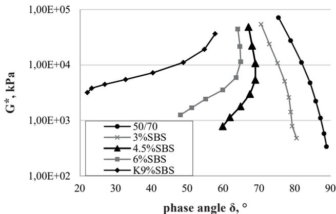
Fig. 6. Black curves of asphalt binders tested at an angular frequency of 10 rad/s in the temperature range of 40–100°C, before ageing by RTFOT method
