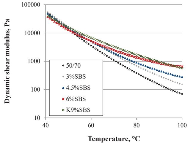
Fig. 2. Temperature dependence of dynamic shear modulus  $|G^*|$  for binders not subjected to RTFOT ageing, at a constant angular frequency of 10 rad/s
