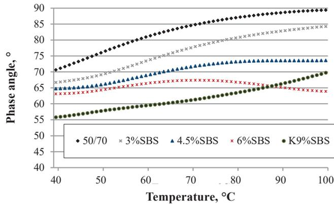
Fig.5. Temperature dependence of phase angle  $\delta$  for binders subjected to RTFOT ageing, at a constant angular frequency of 10 rad/s
