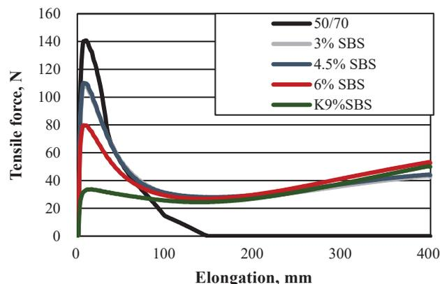
Fig. 14. Mean values of tensile force recorded during the tensile test at the temperature of 5°C for binders submitted to RTFOT ageing
