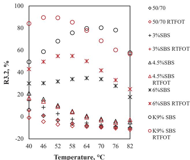
Fig. 12. Compilation of mean percentage values of recovery R3.2 obtained by the MSCR method in a DSR on bitumen samples before and after RTFOT ageing
