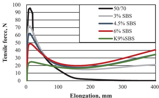
Fig. 13. Mean values of tensile force recorded during the tensile test at the temperature of 5°C
