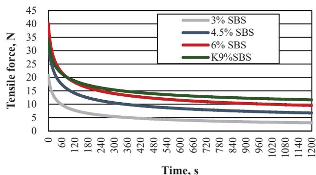
Fig. 15 Relaxation curves of the binders before ageing obtained in the tensile test in a ductilometer at 5°C
