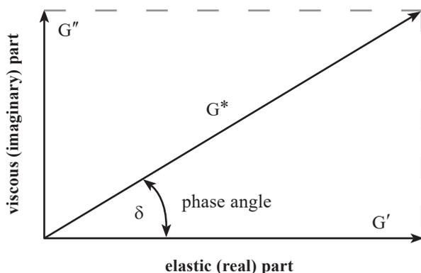
Fig. 1. Graphical interpretation of the complex shear modulus  $G^*$  (based on [1])
