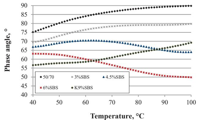
Fig. 3. Temperature dependence of phase angle  $\delta$  for binders not subjected to RTFOT ageing, at a constant angular frequency of 10 rad/s
