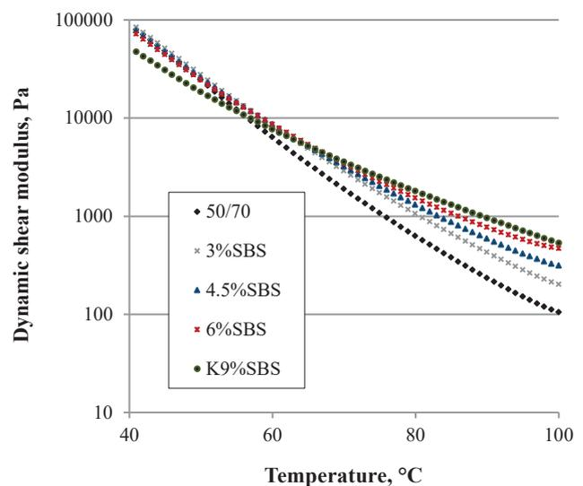
Fig. 4. Temperature dependence of dynamic shear modulus  $|G^*|$  for binders subjected to RTFOT ageing, at a constant angular frequency of 10 rad/s
