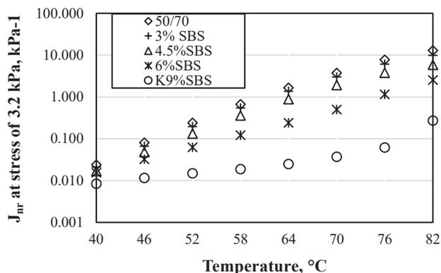
Fig. 11. Values of  $J_{nr}$  at a present stress of 3.2 kPa as a function of the binder temperature after RTFOT ageing
