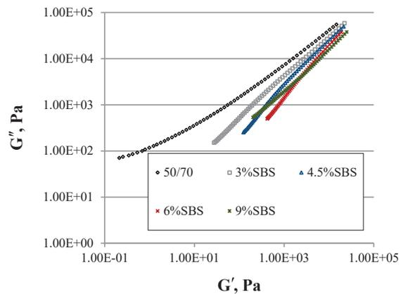
Fig. 8 Cole-Cole diagram of asphalt binders tested at an angular frequency of 10 rad/s in the temperature range of 40–100°C before ageing
