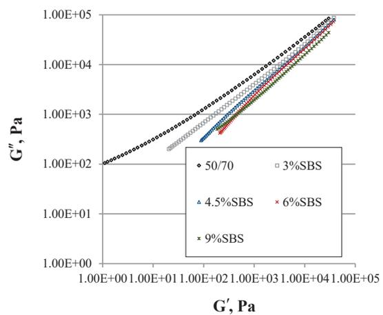
Fig. 9 Cole-Cole diagram of asphalt binders tested at an angular frequency of 10 rad/s in the temperature range of 40–100°C after ageing by RTFOT method
