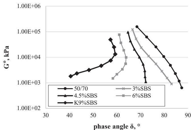
Fig. 7 Black curves of asphalt binders tested at an angular frequency of 10 rad/s in the temperature range of 40–100°C, after being subject to ageing by RTFOT method
