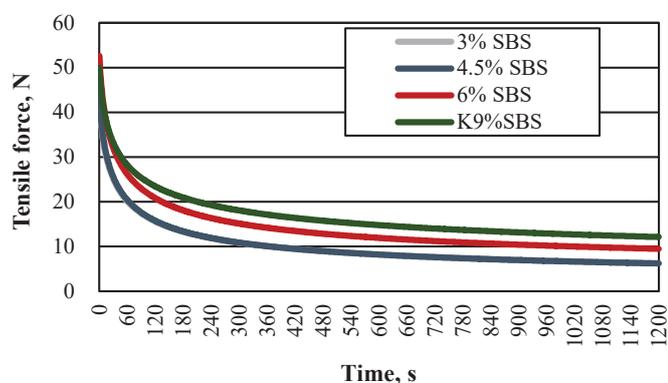
Fig. 16 Relaxation curves of the binders subjected to RTFOT ageing obtained in the tensile test in a ductilometer at 5°C
