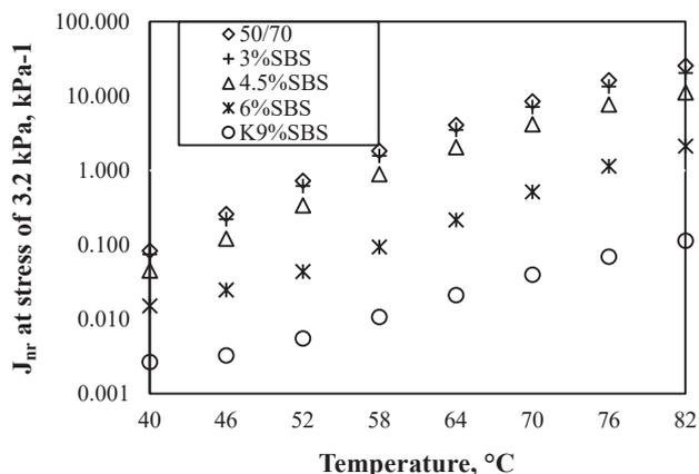
Fig. 10. Values of  $J_{nr}$  at a present stress of 3.2 kPa as a function of the binder temperature before ageing
