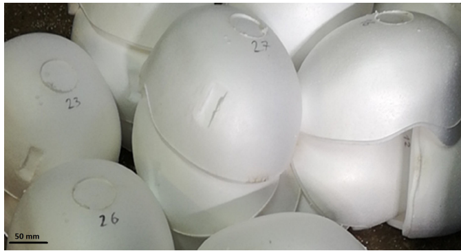
Fig. 3. Finished helmet liners made of EPS
