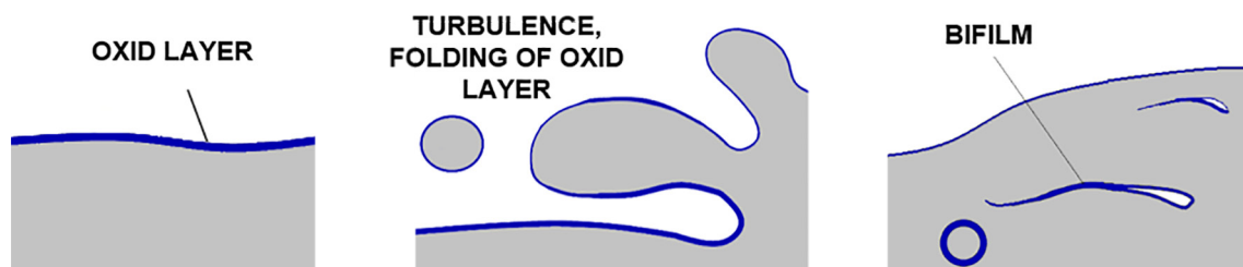
Fig. 1. Scheme of the bifilm origin
