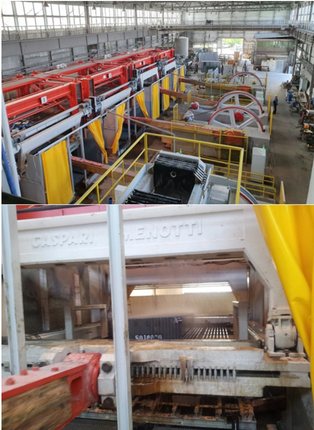
Fig. 6. Gaspari Menotti swing-type steel shot frame saws fitted with a novel diamond bladed frame rising system. Granit-Color Ltd. facilities in Ostrowiec Swietokrzyski [35] (Courtesy of Granit-Color Ltd.)
