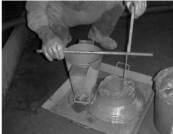
Fig. 3. A slump test showing paste material with 7" slump
