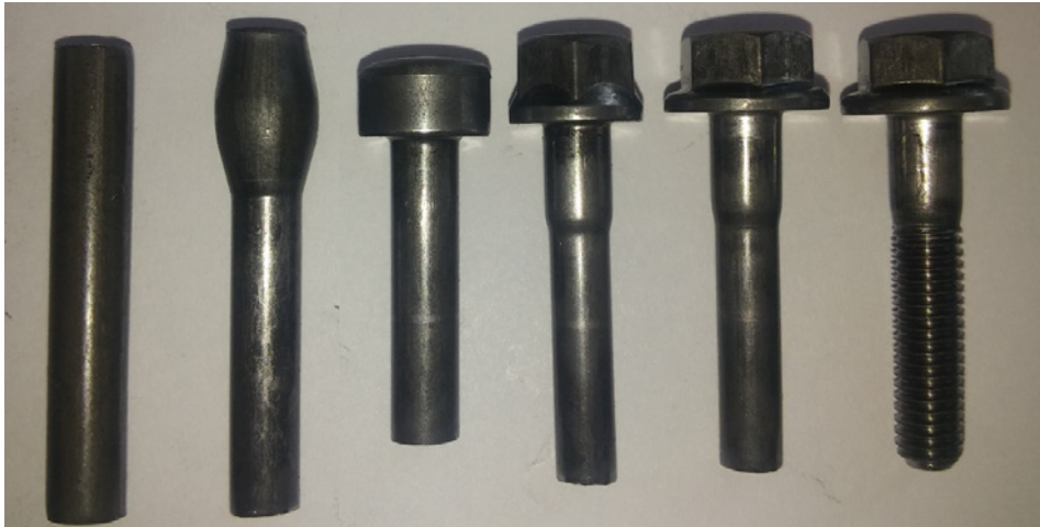
Fig. 3. Wire cut, semi-products and finished bolt with thread
