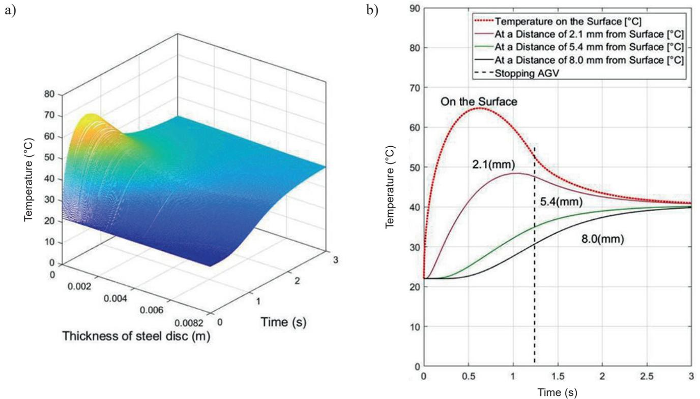
Fig. 10. Organic friction material & steel disc in the thickness of 8.2 mm, load 3020 kg
