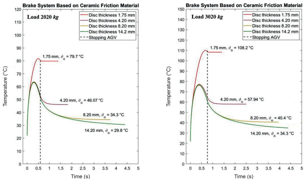
Fig. 7. Temperature course on the disc surface during braking (ceramic friction material)
