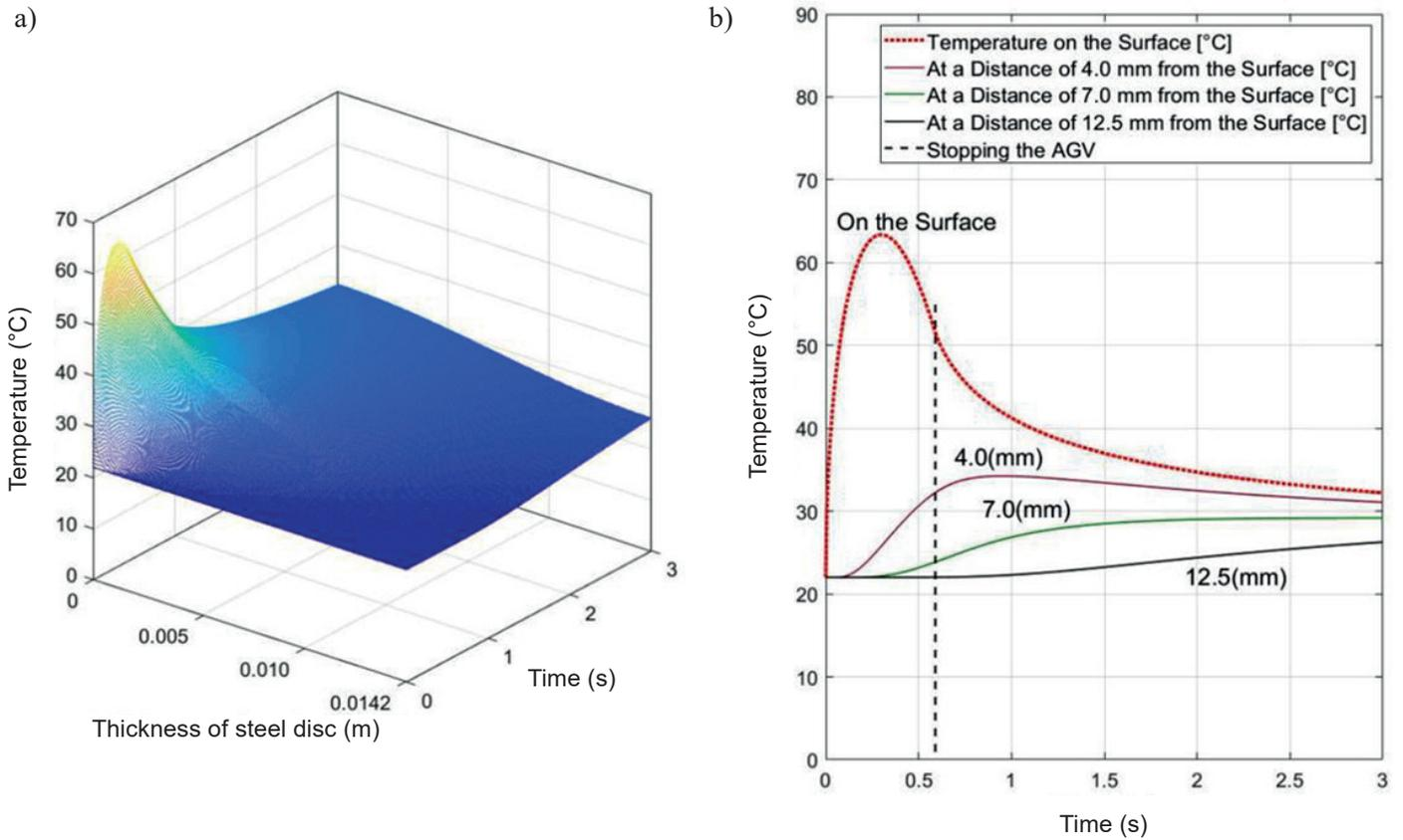
Fig. 11. Organic friction material and steel disc in the thickness of 14.2 mm, load 2020 kg
