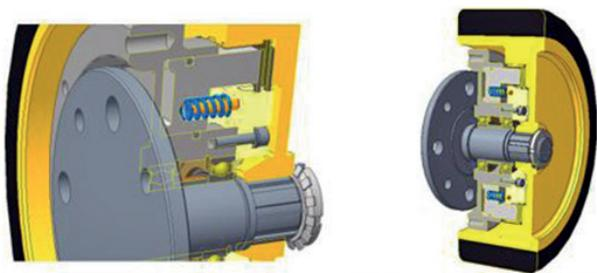
Fig. 1. Concept of drive wheel with integrated multi-disc brake [4, 6]
