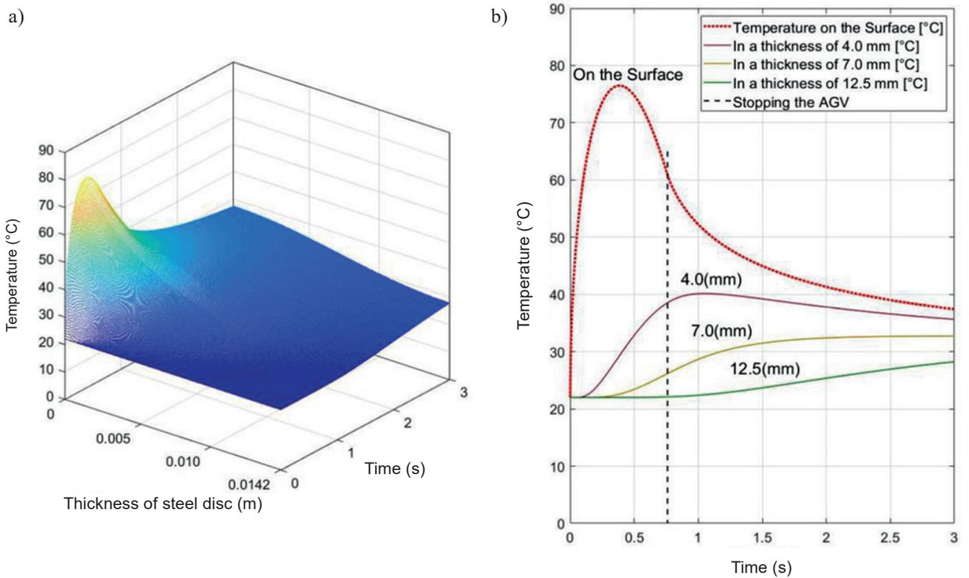
Fig. 12. Organic friction material and steel disc in the thickness of 14.2 mm, load 3020 kg
