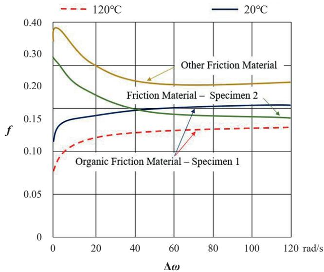
Fig. 2. Coefficient of friction of different friction materials [12]
