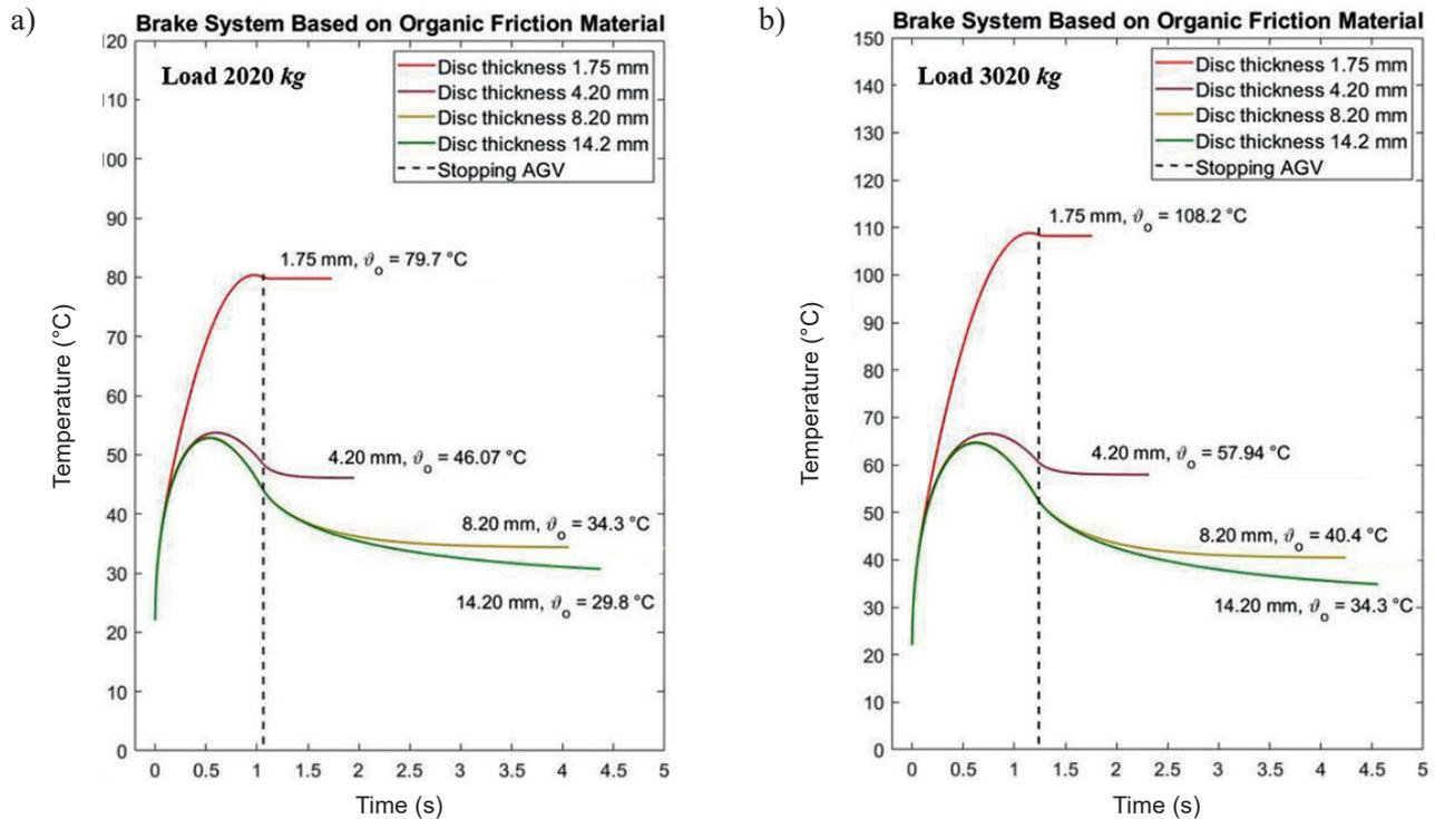
Fig. 6. Temperature course on the disc surface during braking (organic friction material)
