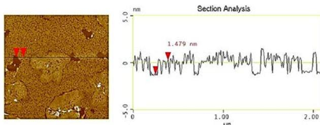
Fig. 3. Section analysis of DA skeletonized layer.
