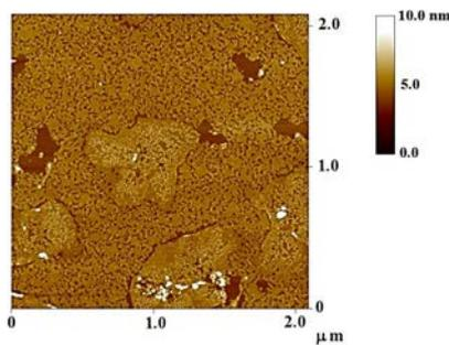
Fig. 2. The AFM image of DA skeletonized layer.
