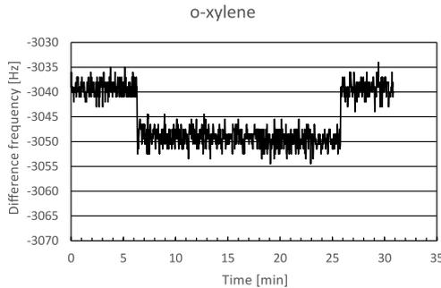
Fig. 7. Interaction of the sensor layer with o-xylene vapors in the air at a concentration of 300 ppm.
