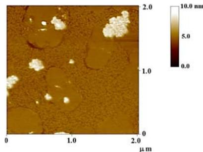
Fig. 1. The AFM image of DA+CA layer.
