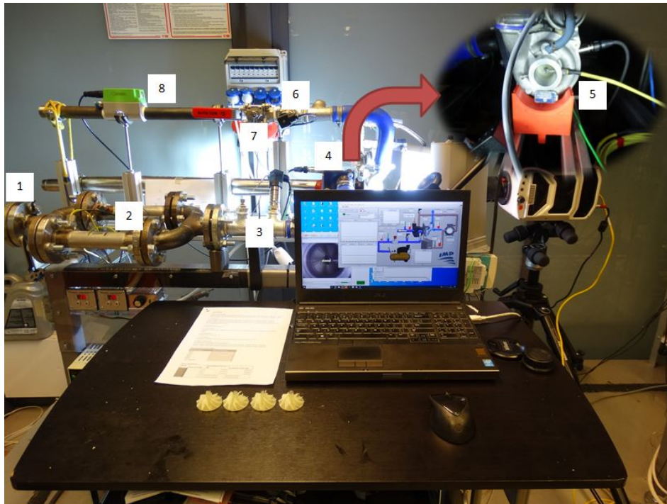
Figure 2: Test stand with a measurement system for registering and determining flow characteristics of turbocharger compressor: 1 – air supply side, 2 – air pre-heated system, 3 and 6 – temperature and pressure sensors, 4 – turbocharger, 5 – speed sensor, 7 – throttle valve, 8 – flowmeter.
