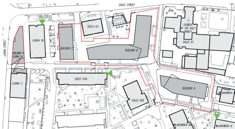
Fig. 1. Site plan of the planned investment and existing neighboring buildings. The outline of the underground part of the new housing complex is marked by a dotted line (own study based on [35]). The location of benchmarks for geodetic measurements is provided - explanations in the text.
