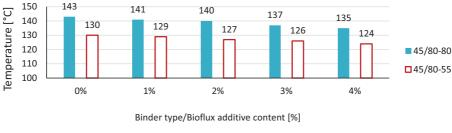
Fig. 6. Compaction start temperature
