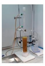
Fig. 1. Ester oxidation reactor
