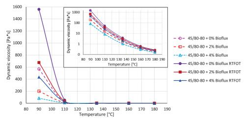
Fig. 2. Dynamic viscosity of original and RTFOT aging PMB 45/80-80 binders
