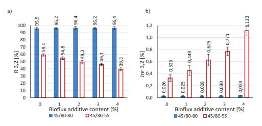
Fig. 8. Comparison of MSCR test results: a) Jnr, b) R
