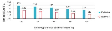
Fig. 5. Binder pumping temperature
