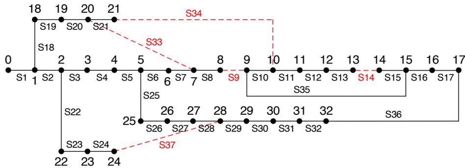
Fig. 9. IEEE 33-bus distribution system after reconfiguration
