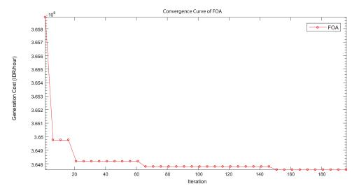
Fig. 4. Convergence graph of the total fuel costs of Sulselbar thermal system
