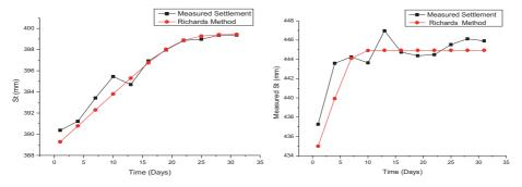
Fig: 2. Measured and predicted settlement values for section K10+900-1
