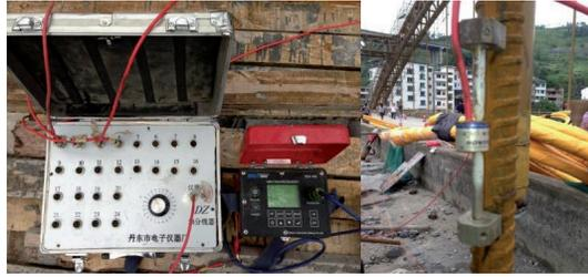
Fig. 6. Temporary derrick internal force monitoring
