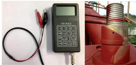
(a) Anchor cable reader (b) Rope meter
