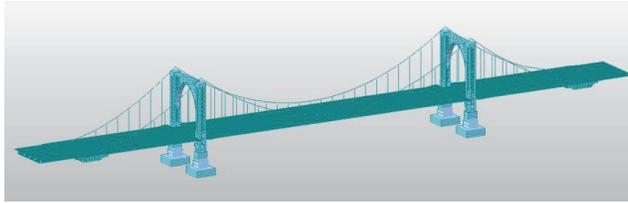
Figure 3: Space plate and shell element model
