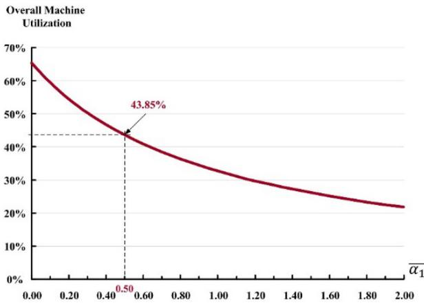
Fig. 5. Impact of differences in  $\bar{\alpha}_1$  on overall machine utilization
