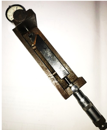
Fig. 11. Device for measuring the dimensional wear of the tip of a cutting tool edge
