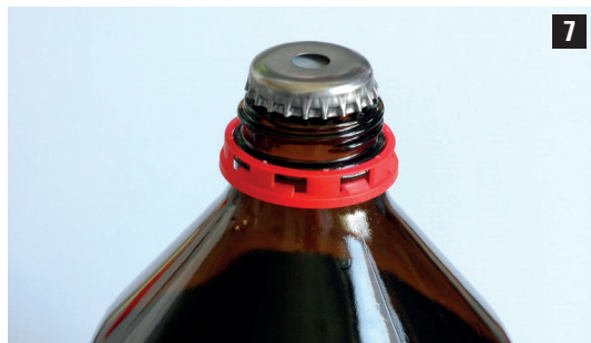
Fig. 7 A bottle closed by a silicone-Teflon membrane (called a septum cap) which protects the contents from humidity and oxygen from the air, enabling reagents to be drawn out with a syringe (the bottle contains anhydrous dimethyl sulfoxide – DMSO)
