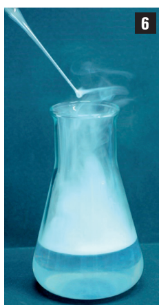
Fig. 6 Reaction of \text{TiCl}_4 with water – note the fog, comprised of hydrolysis products
