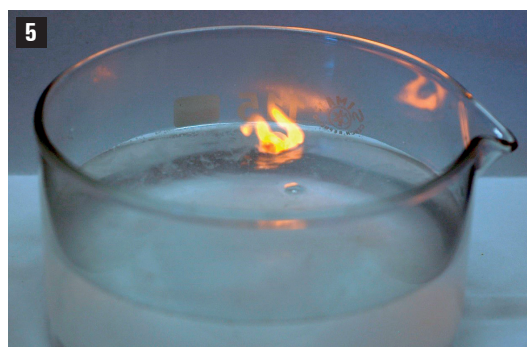
Fig. 5 Metallic potassium violently reacting with water
