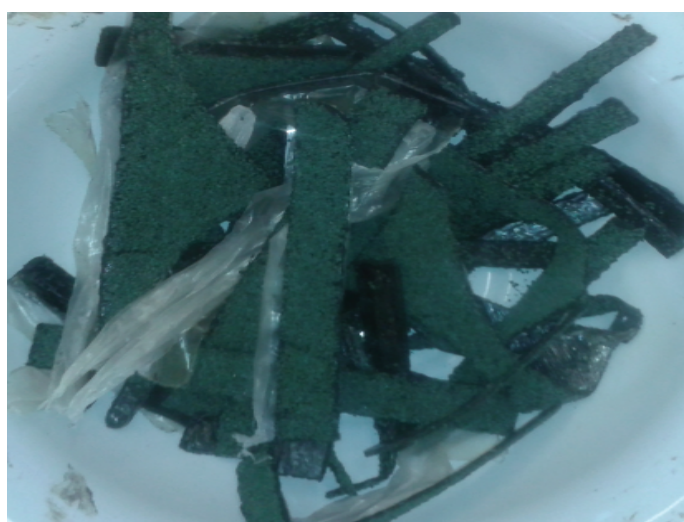
Fig. 1. View of manufacture waste asphalt shingles
