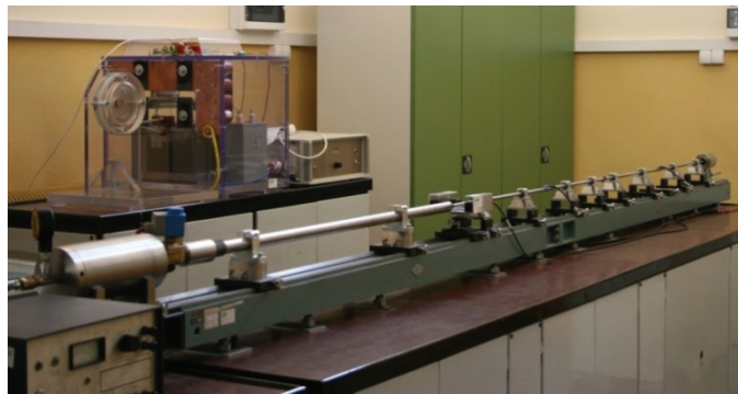
Fig. 2. Hopkinson Pressure Bar set-up for investigation of the material's dynamic behavior [11]
