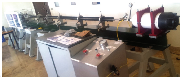
Fig. 4. Gas gun set-up used for perforation tests at high impact velocities and temperatures [8]; a) general scheme, b) photo of the system with the installed thermal chamber
