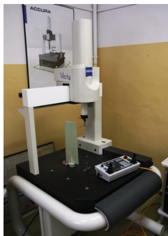
Fig. 3. CNC measuring machine used for plate deformation calculations [11]
