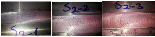
Fig. 4. Surface of the butt joint after the burrs are welded: (a) clamping pitch 30 mm and 1800 rpm; (b) at clamping pitch 60mm and 1800 rpm; (c) at clamping pitch 90mm and 1800 rpm
