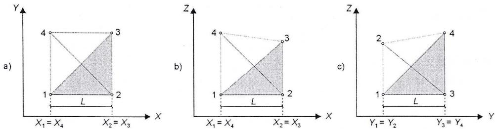
Fig. 2. Projections of a single element of DEM in each plane  $OXY$  (a),  $OXZ$  (b),  $OYZ$  (c).
