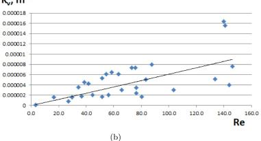
Figure 2: Distribution of experimental points: (a) influence of the Reynolds number (Re) on the descending coefficient of biogas flow resistance for the adhesive bed  $(\zeta_{\varepsilon})$ ; (b) the effect of the Reynolds number (Re) on the gas permeability coefficient  $(K_V)$  of the adhesive bed.
