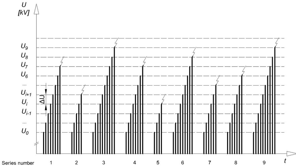
Fig. 2. Example of procedure of an insulation test using the step method.
