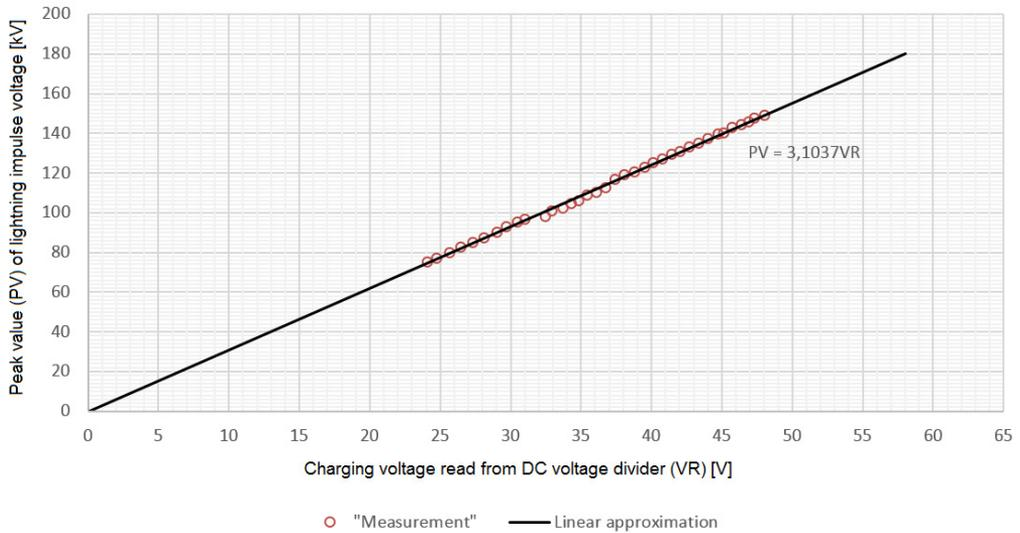
Fig. 5. Generator scaling curve.
