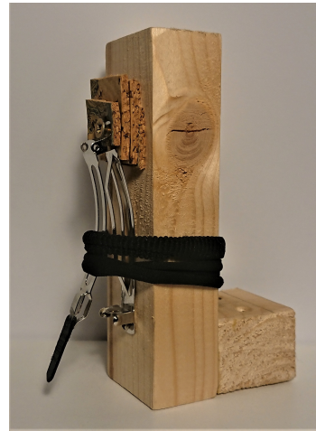
Fig. 4. Plucking mechanism constructed to repeatedly excite the tested string. The cork and elastic bands are used to dampen the springs vibration and make the mechanism quieter.
