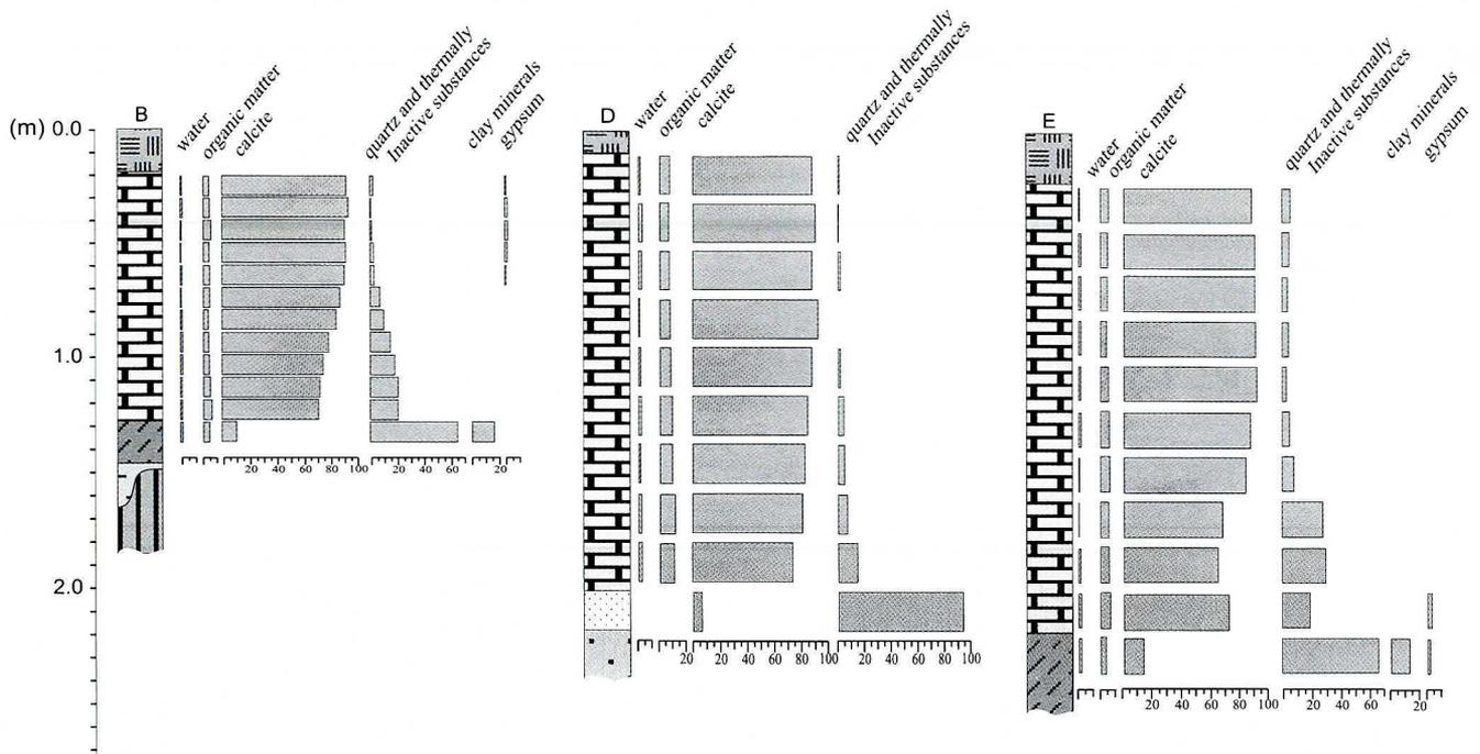
Fig. 5. Composition of studied sediments (in % of dry mass). For key to stratigraphic symbols see Fig. 2.
