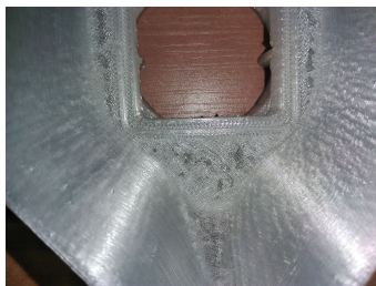
Fig. 10. Most common problems in 3D printing: X or Y axis shift
