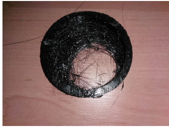
Fig. 1. Most common problems in 3D printing: stringing or oozing
