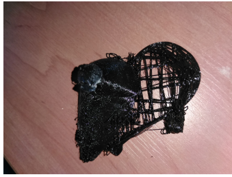
Fig. 8. Most common problems in 3D printing: too thin layers
