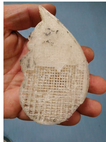
Fig. 7. Most common problems in 3D printing: outer shell not sticking to the inner shell
