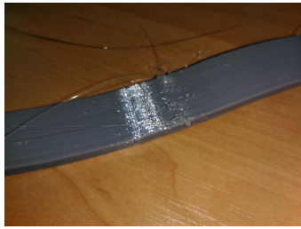
Fig. 2. Most common problems in 3D printing: stringing or oozing
