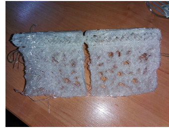
Fig. 5. Most common problems in 3D printing: weak infill
