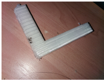
Fig. 9. Most common problems in 3D printing: too high first layers
