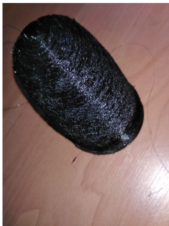
Fig. 3. Most common problems in 3D printing: over-extrusion
