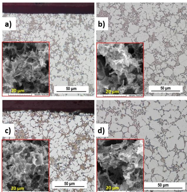
Fig. 5. Microstructure of casting A75 and A90 (OM – etc. Dix-Keller, SEM – etc. HCl); (a) surface area A75; (b) central region A75; c) surface area A90; (d) central region A90
