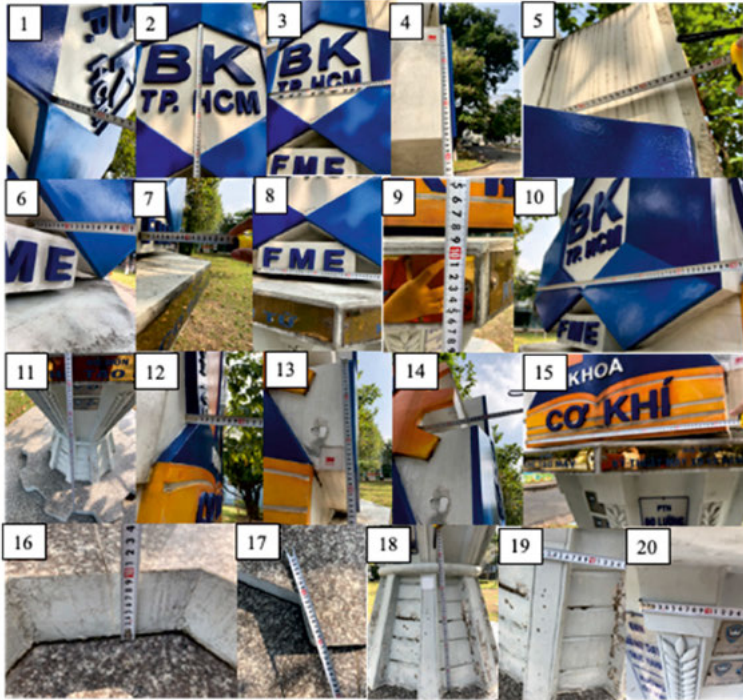
Fig. 4. The direct measurement is performed for determining the size of the object. The ID of each detail is numbered
