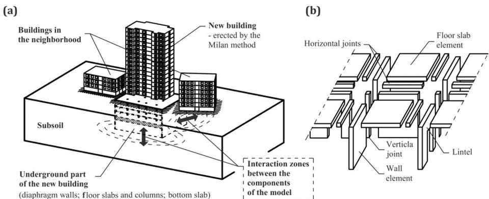
Fig. 1. Components of the interactive and “tracking” model of deeply set buildings together with existing buildings in the neighborhood: a) 3D model view; b) subdivision of the building structure into constitutive elements
