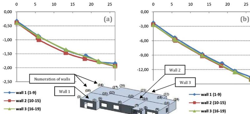
Fig. 10. Building deformation for selected longitudinal walls (numeration of walls given in the picture): a) erection phase; b) occupancy phase
