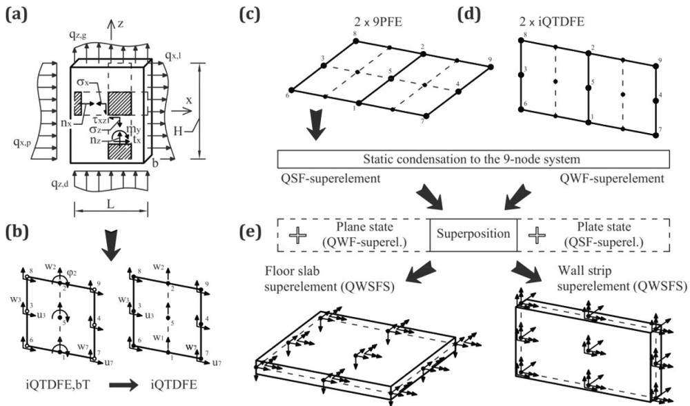
Fig. 2. The developed finite elements: a) element of a wall strip (load diagram and stress state); b) the iQTDfE-element (with/without rotational nodal displacements in the element axis); c–e) manner of construction of the wall-slab QWSF-superelements)
