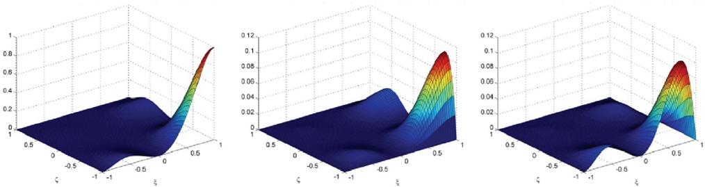
Fig. 3. Graphs of the shape functions for the selected plate (9PF) element nodes: a) graph of  $N_{7v}$  function; b) graph of  $N_{7\varphi_x}$  function; c) graph of  $N_{7\varphi_z}$  function
