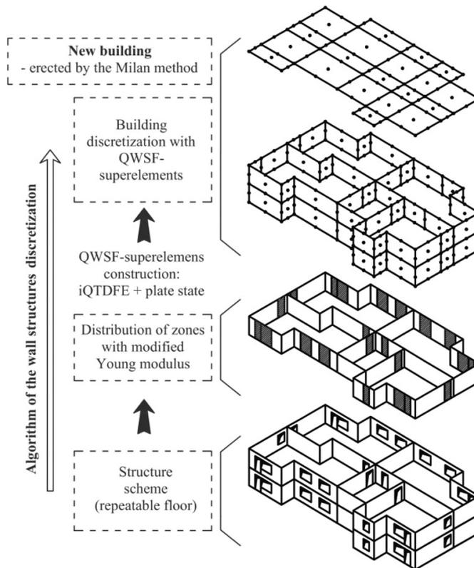
Fig. 6. New building discretization – with the QWSF-superelements – algorithm; Distribution of the iQTDFE-elements with modified modulus of elasticity of concrete
