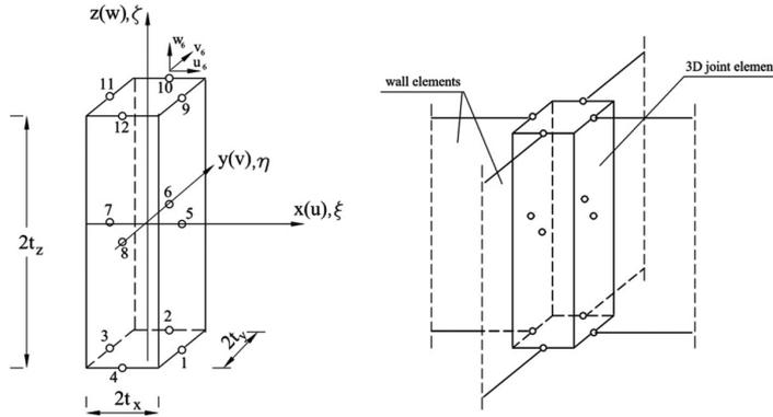
Fig. 4. The 12-node spatial joint element and interconnections between joint element and wall elements
