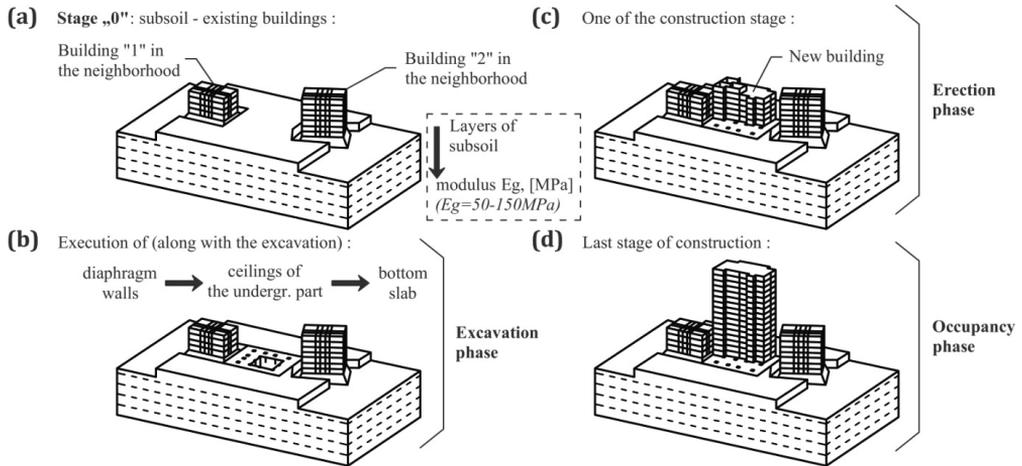
Fig. 7. Exemplary stages of deep foundation building erection (descriptions in the figure)
