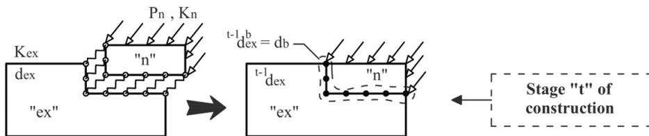
Fig. 8. Scheme of adding computational block (placement area) from the global FE system according to the developed “tracking” model
