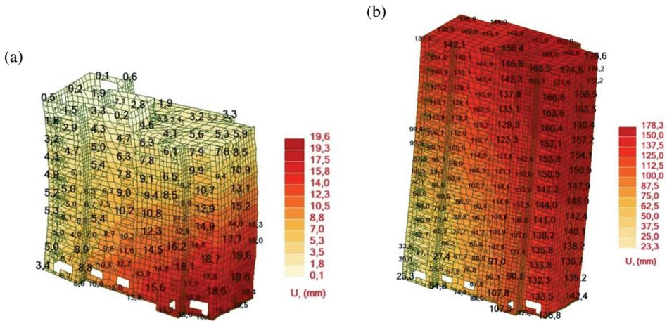
Fig. 9. State of deformation of the new building in selected stages of erection (deformation maps of the system based on the transformed kinematic constraints – obtained according to the “QFEM + tracking model” method): a) erection phase (one of the construction stage); b) occupancy phase (last stage of construction)
