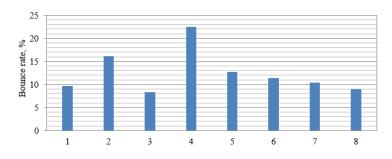
Figure 2: Failure diagram of steam turbines parts: 1 – flow part; 2 – bearings; 3 – oil system; 4 – regulation; 5 – steam distribution; 6 – pipelines and fittings; 7 – other elements; 8 – failures without damage.
