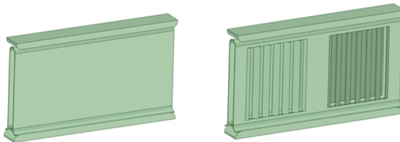
Figure 7: Geometrical model: plain fin (left picture) and louvered fin (right picture).
