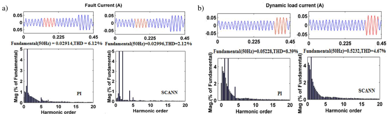
**Fig. 8.** Simulated result of THD analysis of PI and SCANN Load current
