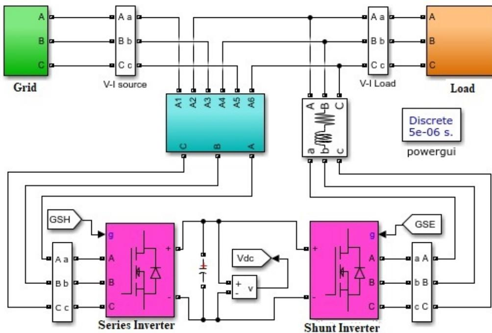
Fig. 5. UPQC simulation model
