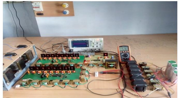
Fig. 10. The hardware setup of SCANN based UPQC
