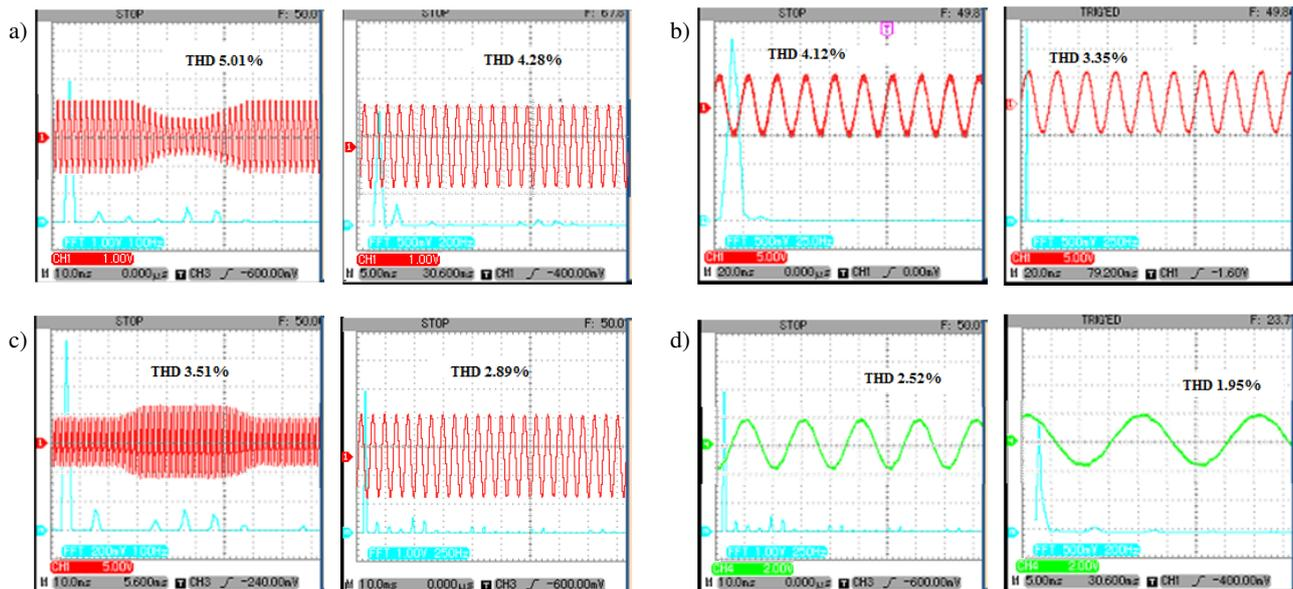
**Fig. 11.** Sag and Swell load voltage and current: (a) sag source voltage and sag load voltage, (b) sag source current & sag load current, (c) swell source voltage & swell load voltage, (d) swell source current and swell load current
