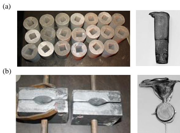
Fig. 1. (a) Example view of the test rod moulds and of a test rod; (b) Example view of the metal moulds for casting chemical analysis specimens and of a chemical analysis specimen
