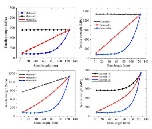
Fig. 4. Functionally graded materials tensile strength from distal to proximal
