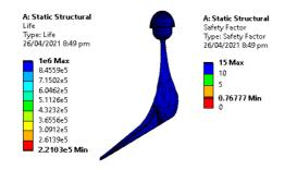
Fig. 10. Fatigue life and factor of safety
