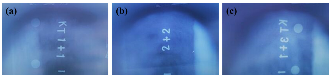
Fig. 1. X-ray inspection of hardfacing layer: (a) UMCo50, (b) ST1, (c) ST6
