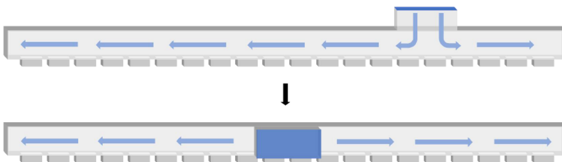
Fig. 13. Schematic diagram showing the air inlet position adjustment
