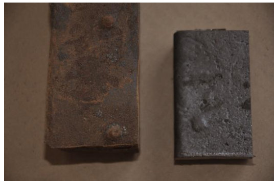
Fig. 12. Ductile iron casting surface. On the left side, a casting made in the “in-mold” technology. On the right, the casting surface is made in the traditional sandwich spheroidization method
