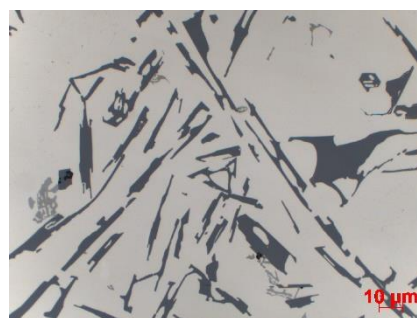
Fig. 7. The morphology of eutectic silicon in the central part of casting, 1000x magnification; ablation mould
