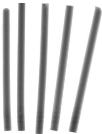
Fig. 4. X-ray images of tensile test bars
