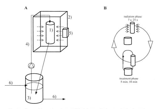
Fig. 1. A – diagram of the experiment layout: 1) biological reactor, 2) microwave chamber, 3) retention reservoir, 4) sewage supply to the reactor, 5) microwave generator, 6) sewage replacement in the retention reservoir; B – diagram of the operation of the experiment arrangement
