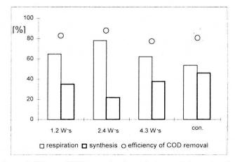
Fig. 2. Dependence of efficiency of COD removal and participation respiration and synthesis in this process on microwave amount
