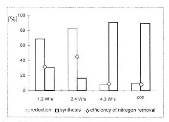
Fig. 3. Dependence of efficiency of nitrogen removal and participation reduction and synthesis in this process on microwave amount
