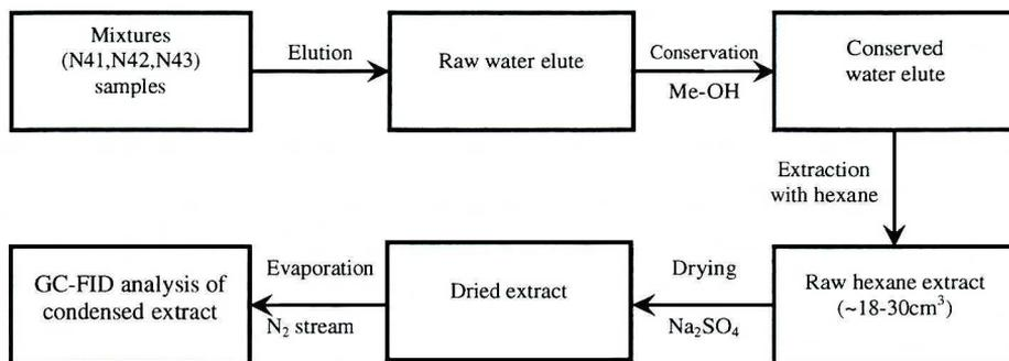
Fig. 1. Mixture elution experiment scheme
