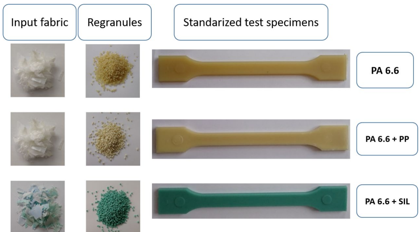
Fig. 3. Standardized test specimens obtained in accordance with ISO 294
